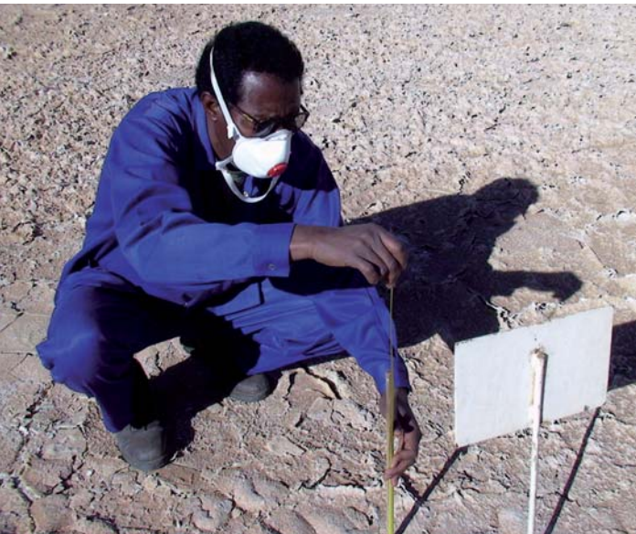
Bi-annual Relative Stability Measurements of a Mill Tailings Impoundment.
